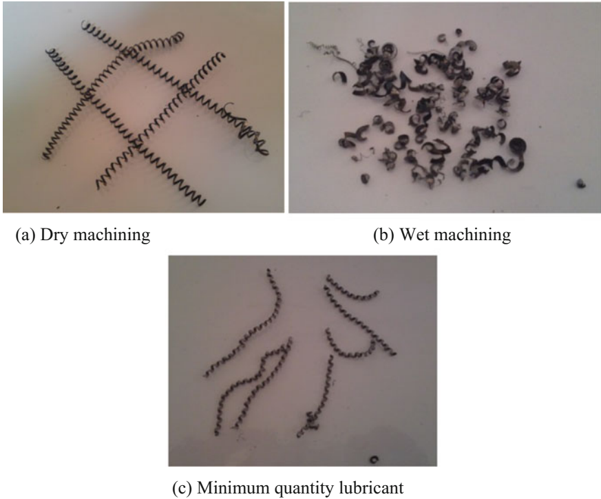
Fig. 3 Chip formations for light turning operation
