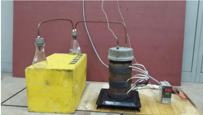
Fig. 4 Experimental setup of the pyrolysis process
