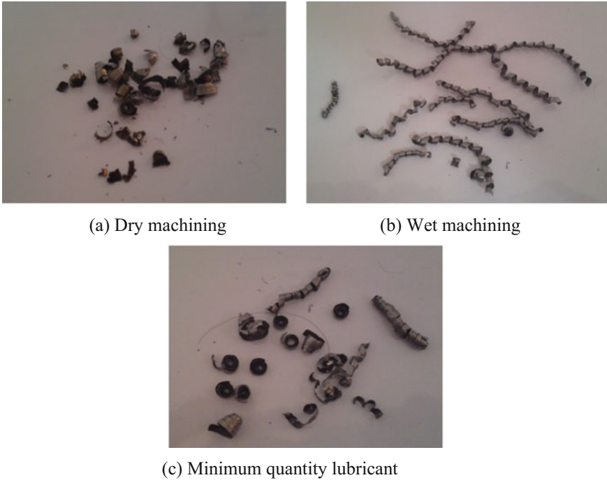
Fig. 2 Chip formations for medium turning operation
