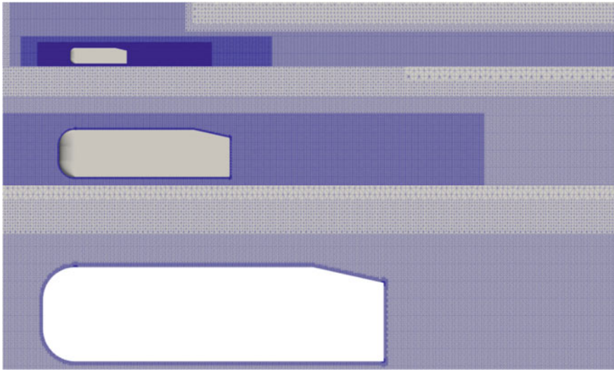
Fig. 4 Slice at z = 0 for the mesh used on the Ahmed body. Three different zoom ratios
