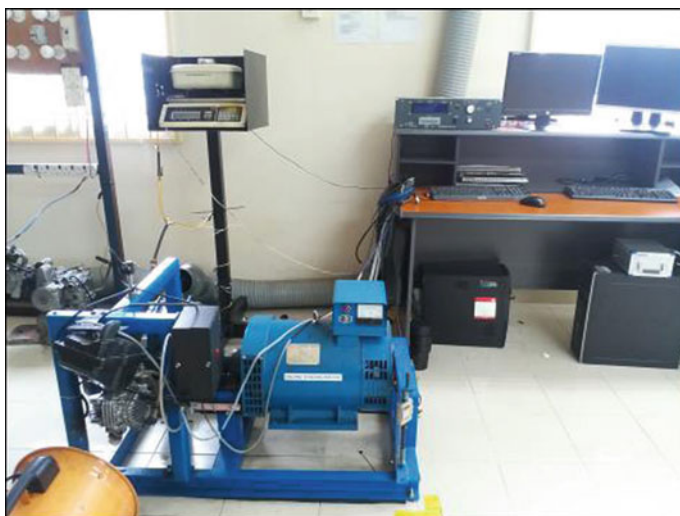
Fig. 1 Experimental setup for gasoline engine performance measurement
